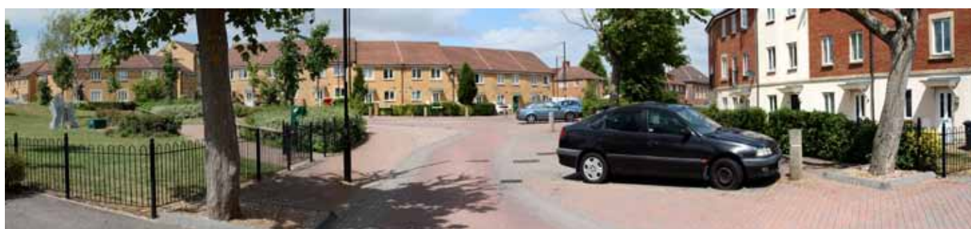
40. Highways should be designed to allow young children access to open and play spaces without parental supervision. Recent guidelines in Manual for Streets are being implemented to allow this to happen. The above examples show shared space solutions.
